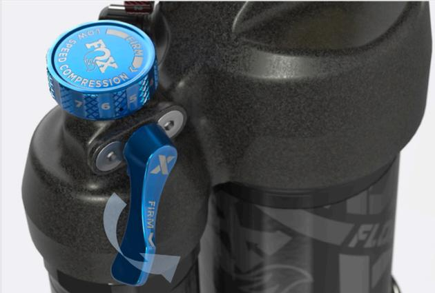
Turn the 2-position Compression lever to the fully **OPEN** mode (counter-clockwise).
