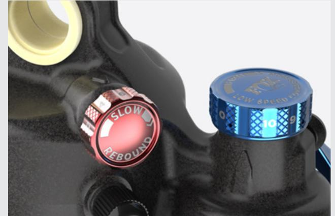
Turn the Rebound adjuster [red] and the Compression adjuster [blue] all the way to the closed position (full clockwise).
