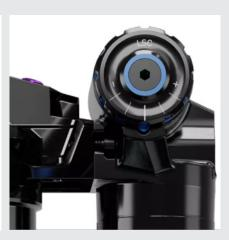
Turn the Rebound adjuster [red ring] all the way to the closed position (full clockwise). Set the compression adjusters [blue rings] to their middle positions.
