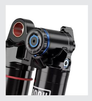
Turn the lock-out lever to the fully OPEN position (counter-clockwise).
