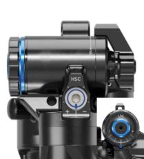
Turn the Rebound adjuster [red ring] all the way to the closed position (full clockwise). Set the compression adjusters [blue rings] to their middle positions.
