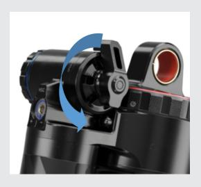
Turn the lock-out lever to the fully **OPEN** position (counter-clockwise).
