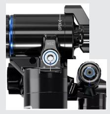
Turn the Rebound adjuster [red ring] and the Hydraulic Bottom Out (HBO) [purple adjuster] all the way to the closed position (full clockwise). Set the compression adjusters [blue rings] to their middle positions.
